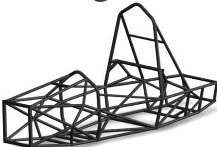
Design of Formula Student Frame using FEA (O. Polívka, 2023)
