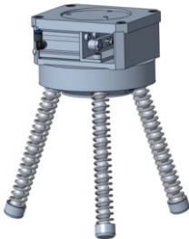
SOFT grippers for non-engineering applications (M. Mařík, 2023)
