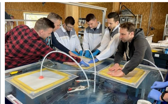
Infusion lamination of composites by students of FME in cooperation with Fraunhofer-IWU (Zittau, Germany)
